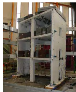
Dynamic torsion behavior of RC building International benchmark SMART 2013
